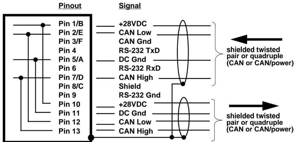
Note: The RS-232 lines defined for this connector type are optional and may be used for device programming, configuration, etc. They have no relationship to CAN or CANaerospace.
