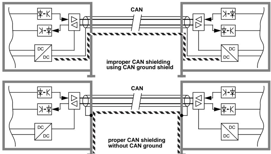
Strongly encouraged is the use of optically isolated CAN interfaces for all units in the network. For the wiring, AWG 22 aerospace standard shielded twisted pair (STP) or shielded twisted quadruple (STQ) should be used.
